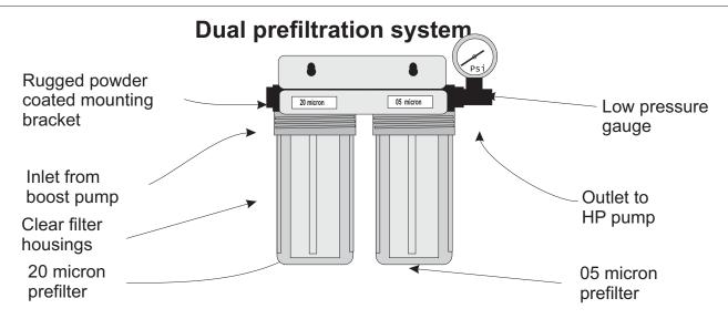
5" x 10" FDA approved polypropylene housings are heavy duty industrial rated at 125 psi. O-ring sealed to provide leak free operation. Standard 3/4" FNPT inlet and outlet.
