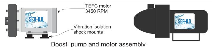
High Head poly pump with closed impeller close coupled to 3450 RPM 1/2HP motor provides 15-20 psi of boost pressure for optimum filter life.
