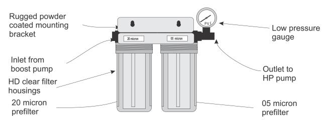
5" x 10" FDA approved polypropylene housings are heavy duty industrial rated at 125 psi. O-ring sealed to provide leak free operation. Standard 3/4" FNPT inlet and outlet.
