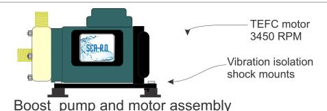
High Head Magnetic Drive poly pump close coupled to 3450 RPM motor provides 20-25 psi of boost pressure for optimum filter life.
