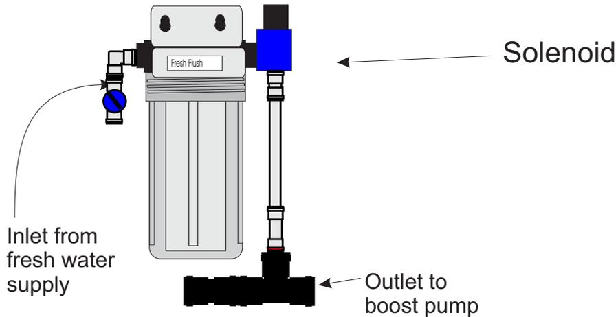
Auto Flush option flushes system on every shut down with de-chlorinated fresh water to purge sea water from system and greatly extend membrane performance.
