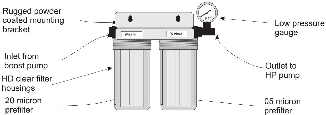
5" x 10" FDA approved polypropylene housings are heavy duty industrial rated at 125 psi. O-ring sealed to provide leak free operation. Standard 3/4" FNPT inlet and outlet.
