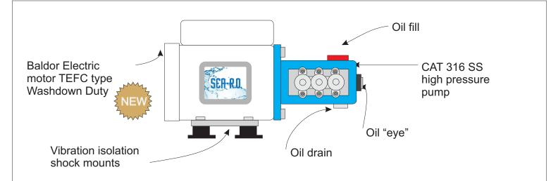
High pressure pump and motor assembly
