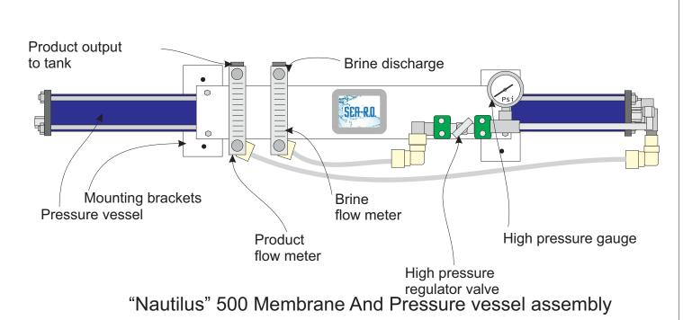
Pressure vessel is all fiberglass construction, 1000 psi rated. Simplified end cap design is rugged and easy to service with no special tools required, pressure and product ports are 316 SS with o-ring seals that allow fittings to swivel and eliminate stress on end cap material. Industry standard membrane size is available worldwide.
