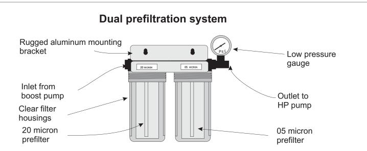
Clear FDA approved polypropylene housings are heavy duty industrial rated at 125 psi. O-ring sealed to provide leak free operation. Standard 3/4" FNPT inlet and outlet.
