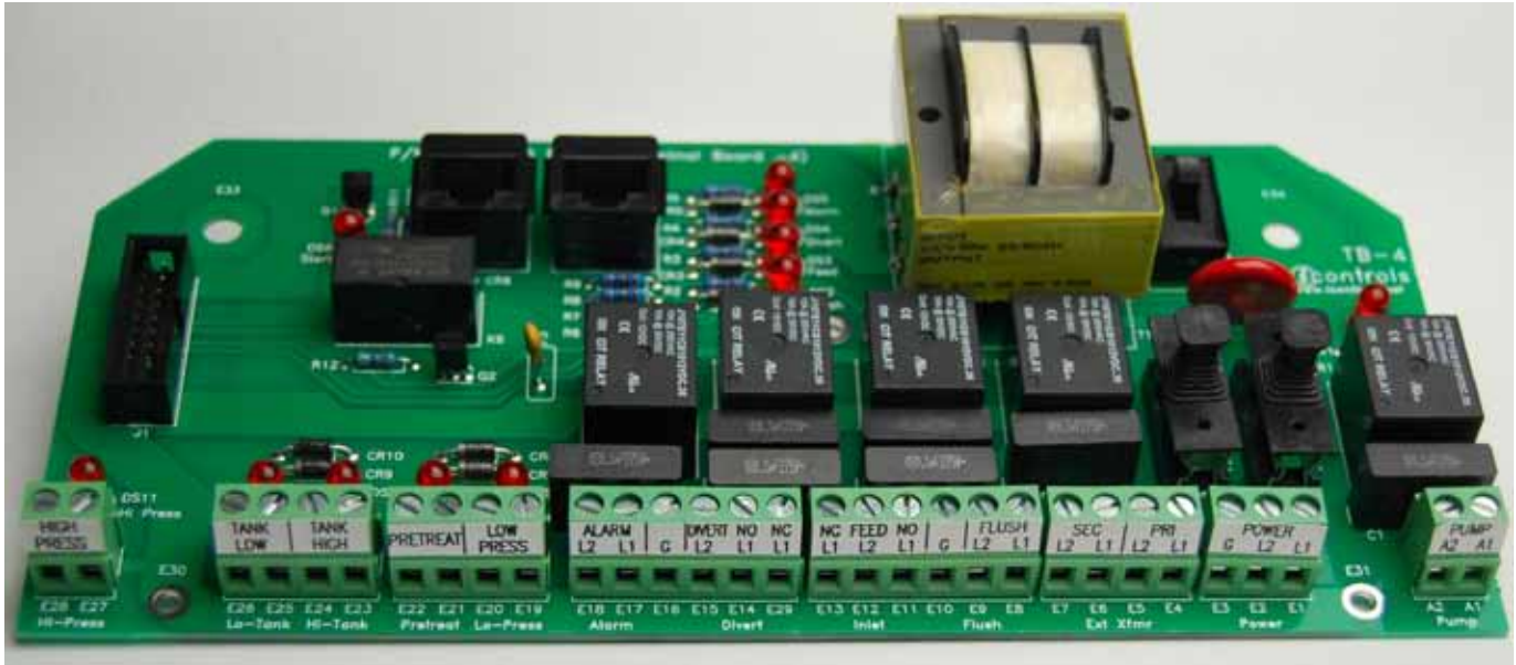
Figure 4. Controller Detail: Terminal Board, TB-4 (See Fig. 1 for schematic)
